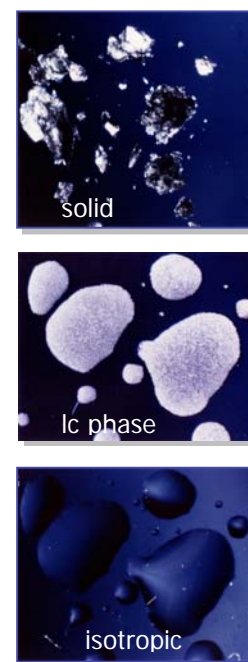
Fig. 1. Behavior of a liquid crystal as temperature increases (top to bottom).
