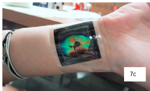
Fig. 7. Manufacture of a cholesteric lc temperature patch.
